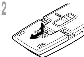
2 Lightly press down on the arrow and slide the battery cover open.
