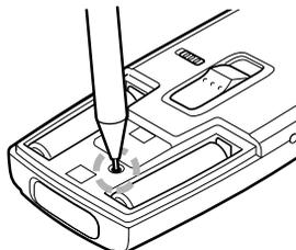
If the display or the recorder acts strangely, lightly press the reset button in the battery compartment with the tip of a ballpoint pen or a similar object.
