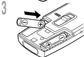
3 Insert two AAA alkaline batteries, observing the correct polarity.
