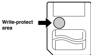
Attach the write-protect seal to the write-protect area to prevent valuable data from being erased accidentally.
